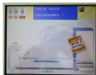
Fig. 18: Example for MP 12N: Operating panel input window display
