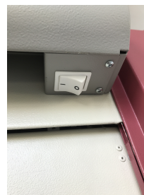
Fig. 14: On/off switch for antiglare lighting
