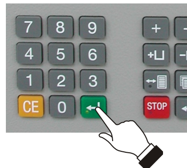
Fig. 18: Example for MP 12N: Operating panel "Return" key
