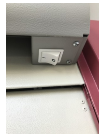
Fig. 15: On/off switch for antiglare lighting
