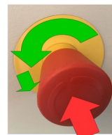
Fig. 8: Pressing/disengaging the emergency stop button
