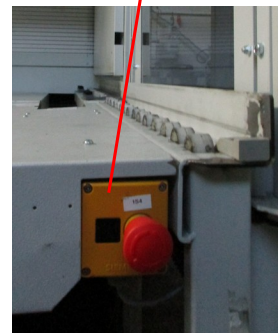
Fig. 30: Automatic drawer with main switch on the left side of the lift and emergency stop button on the right side of the lift
