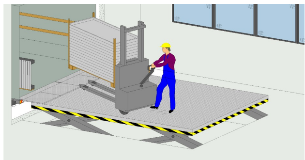
Fig. 25: Unloading with powered auxiliary equipment using a loading ramp Container transport for lift width > 3260 wit forklift in longitudinal direction of containers
